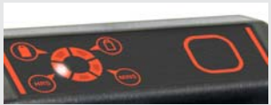
Two button presses on-load activates the time display. The 'HRS' LED flashes twice.
