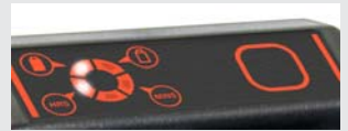
The number of hours is indicated by the number of lit LEDs: 1 LED = 1 hour.
